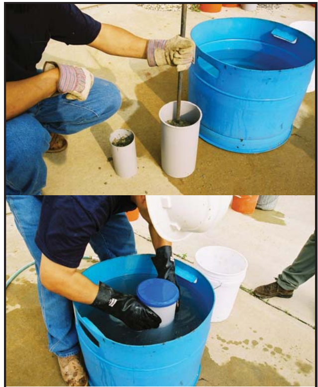
Making and Curing Cylinders in the Field
